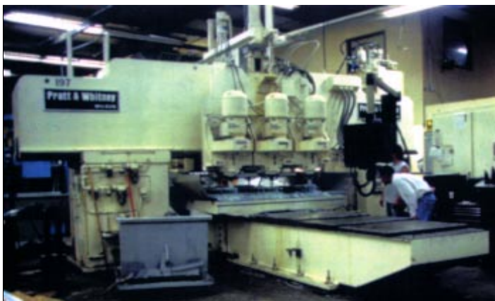
NCCS' PostWorks product can easily be configured to produce code for the complex machines used at L&S, such as this multi-spindle Pratt & Whitney mill.
