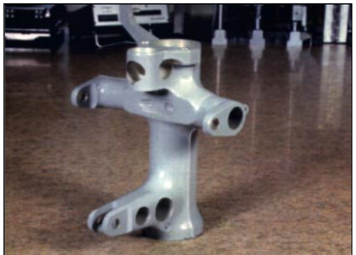
A complex aircraft part that required multi-axis machining was programmed using NCL.
